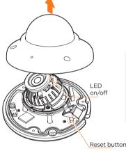
Resetting the camera: To reset the camera's settings, including the network settings, use the tip of a paper clip or a pencil. Press the reset button for five (5) seconds.
