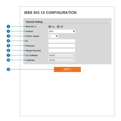
The feature is needed when connecting the camera to a network protected by the IEEE 802.1X.
