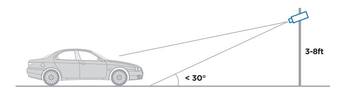
THE CAMERA SHOULD BE MOUNTED AT AN ANGLE NO GREATER THAN 30 DEGREES
