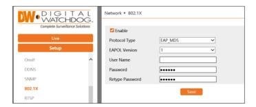
Connect the camera to a network switch that supports 802.1x protocol. The switch can be treated as an authentication system to find the device in a local network. If the camera connected to the network interface of the switch has passed the authentication of the switch, it can be accessed via the local network.
