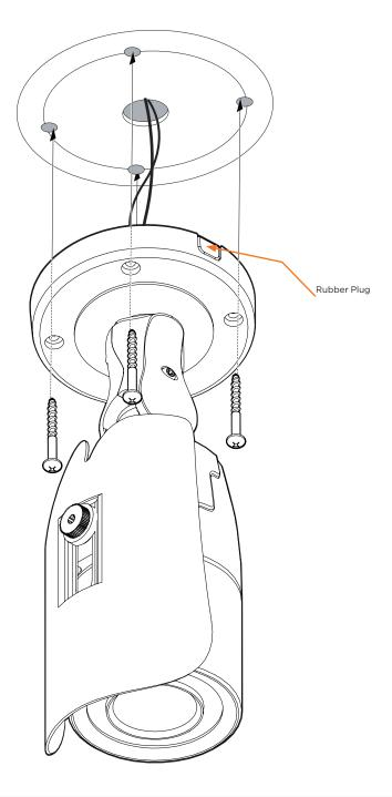
NOTE: Remove the rubber plug on the side of the camera's bracket and use the gap as a cable guide to prevent cables from getting caught between the camera and the mounting surface.
