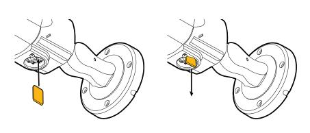
NOTE: Maximum SD Card size supported: Up to 1TB micro SD / FAT32. When inserting the SD card into the card slot, the SD card's contacts should be facing upward, as shown in the diagram.
