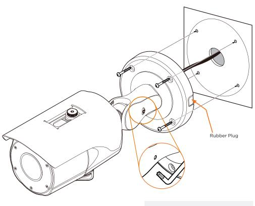
NOTE:Based on the installation, remove the rubber plug on the side of the camera's bracket for a cable guide to prevent cables from getting caught between the camera and the mounting surface.
