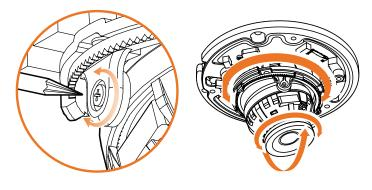
5. When assembling the dome back on the camera, align the screw holes in the dome and the camera's base.
