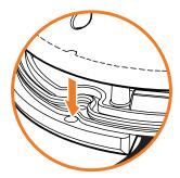
6. When the installation is complete, remove the inner protection film and dome's protective film. Softly wipe the dome/lens cover with lens tissue or a microfiber cloth with ethanol to remove any dust or smudges left from the installation process.
