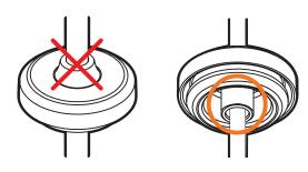
**NOTE:** Bending the cable may cause water leakage.
