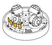
**NOTE:** Maximum SD Card size supported: Up to 1TB micro SD / FAT32. When inserting the SD card into the card slot, the SD card's contacts should be facing upward, as shown in the diagram.
