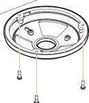
NOTE: Cables with ø4.5mm to ø5.5mm thickness should use the black rubber ring. Cables over ø5.5mm in thickness should use the white rubber ring.
