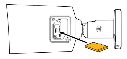
NOTE: Maximum SD Card size supported: Up to 1TB micro SD / FAT32. When inserting the SD card into the card slot, the SD card's contacts should be facing upward, as shown in the diagram.
