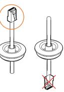
Once the network cable is passed through the grommet: a. Insert the grommet into the bottom of the camera base.
