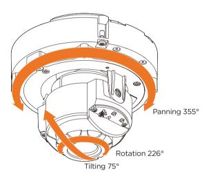
NOTE: When setting up the camera for the first time, use the CALIBRATE button on the camera's web GUI to auto calibrate the camera's lens before operation.
