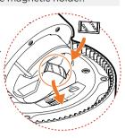
WARNING: The moisture absorber prevents moisture buildup inside the camera, which may cause image performance issues and damage the camera.
