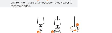
NOTE: When using the waterproof cap, crimp the RJ45 connector after passing the
