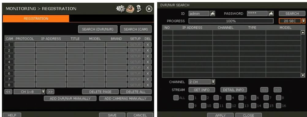
The module will scan the network for all supported DVR/NVR automatically. Select the DVR/NVR you wish to register from the search results and press the 'GET INFO' button to obtain the device's streaming profile. 'DETAIL INFO' allows you to get more information on the device's streams. If necessary, enter the user ID and password for the device you are registering. You can also select which channels from the DVR/NVR you wish to register. Click 'APPLY' to register the device.
