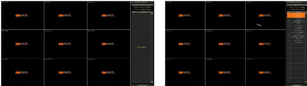
2. Select the camera in the list and drag and drop it to the channel you want to assign to the camera. (While moving, the mouse pointer is changed to
