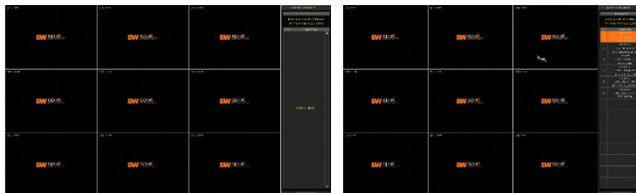
6. Select a camera and while clicking on the camera, drag it to a channel to assign it. If needed, enter the user ID and password for the device you are registering.
