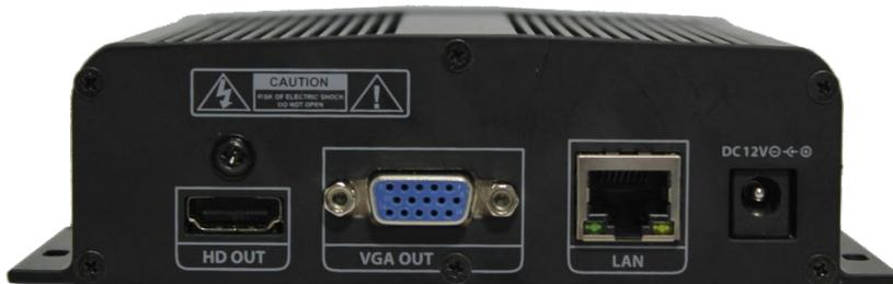
1. HD out: Connect a true HD monitor to the unit (cables not included).
